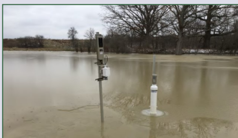
Water level recorders at one project site
